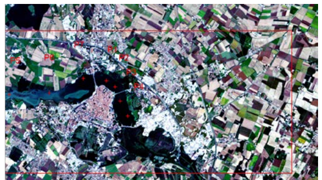
Figure 4. OLI scene (subset) Lake Mantua (Italy): OLI scene from September 23, 2014 with 7 in-situ measurement points.
