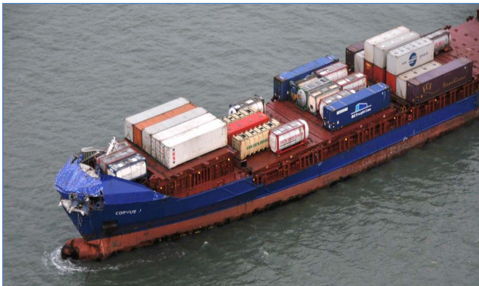
Figure 8 : Corvus J with severely damaged hull after collision with the Baltic Ace (6/12/2012).
