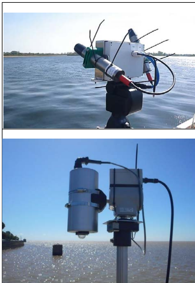
Figure 1. (a-top) PANTHYR radiometer system, (b-bottom) HYPSTAR® radiometer system. Cable tie spikes are used for bird avoidance.
