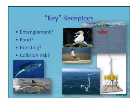
Entanglement tension leg structures have taught mooring lines. – simple structures (point to top right) unlikely. More complex structure (point to bottom right) maybe....but a lot of things have to go wrong first. Ultimately we don't have enough/any data to support entanglement.
