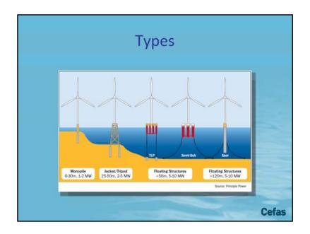
120+ spar buoys look like a good option. UK doesn't have much water this deep so unlikely to see (m)any of these 75-120 semi-subs. Few areas suitable. However, in shallow UK waters means the area taken up by mooring lines could be quite large
